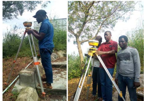
Figure 2. Data Acquisition on Control Point (base point) at Eleyele Hill.
